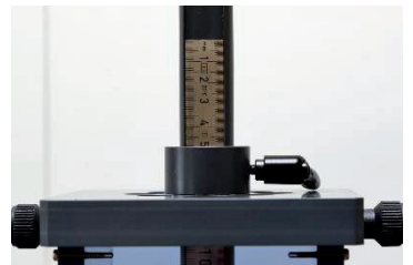
Thickness measurement of sample, holding table fixed with toggle screw
