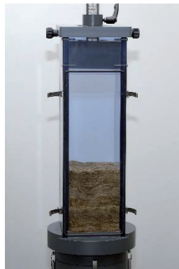
Receptacle with tensioning piston and toggle screw
